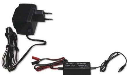
Mains feeder AM240 and converter for battery AM140
